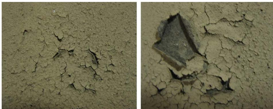
Fig. 10. Image of the coated surface of catalyst prepared by CP at 80 °C (left) and by SP at 80 °C (right).
